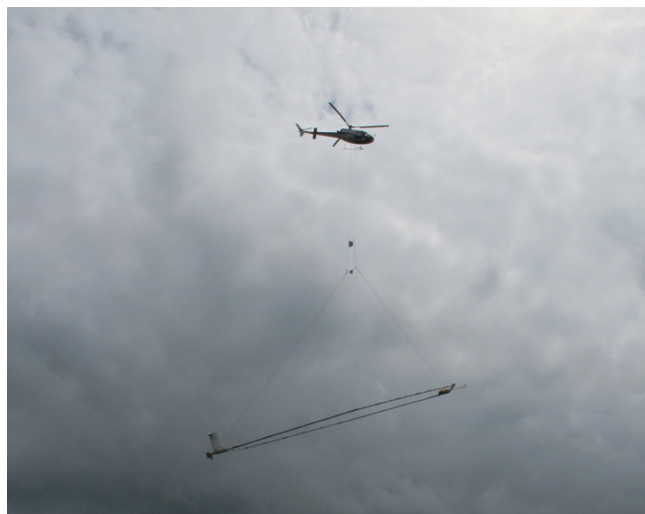
Figure 4-4: Photo of the SkyTEM304M system in suspension beneath the helicopter.
